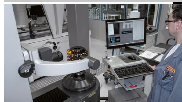
»hobCheck 800« from ZOLLER in action during quality control at SANDVIK Tooling Supply Schmalkalden.
