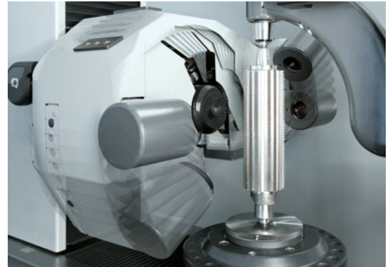
Swiveling optical carrier for distortion-free imaging of tooth profiles.
