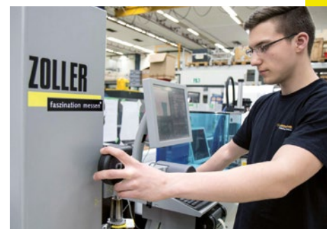
CNC-controlled tool presetting and measuring machine ZOLLER »venturion 450«.
