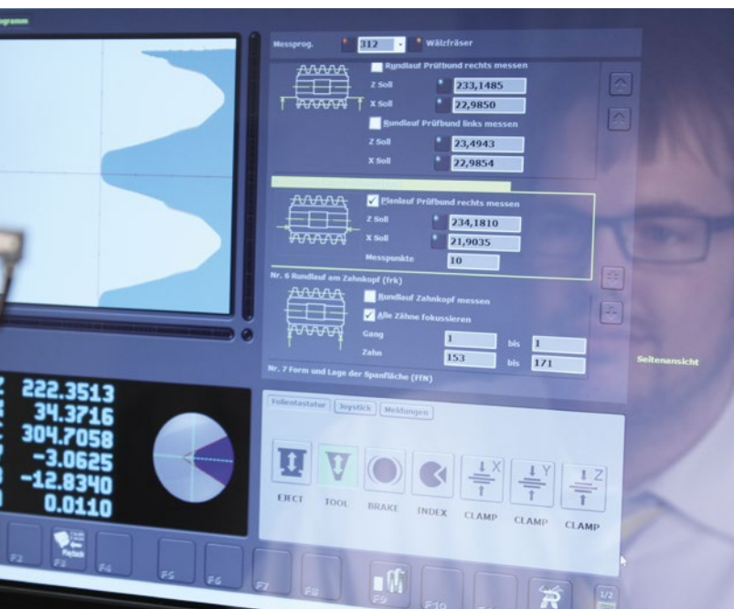
User-friendly image processing system »pilot 3.0« with fully automatic calculation of the quality classes and graphic documentation.
